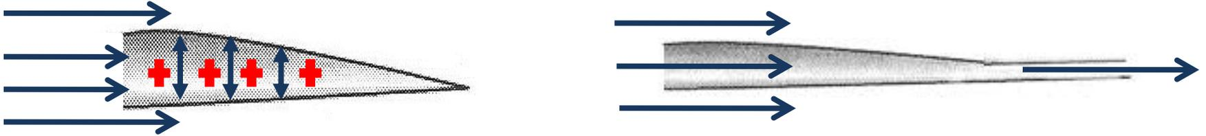
**If the air inside the cell is allowed to escape then the cell cannot maintain its aerodynamic shape**
